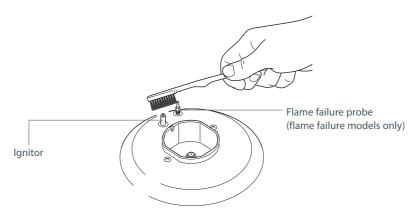
Fig.15 Cleaning the ignitor and probe
